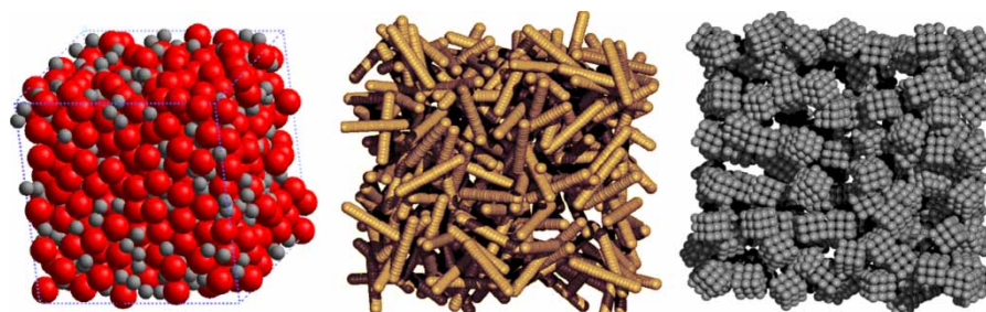
Figure 8. Examples of particulate systems which can be modelled using a combination of DPD thermostat and the spherical subdivision description of particle shape, from left to right: binary sphere mixture, fibres, and cuboids.
